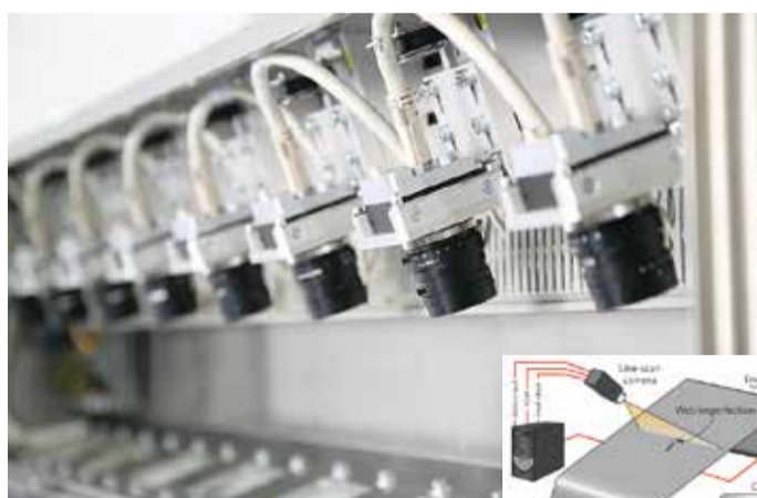
Camera based monitoring systems that perform 100 % checks of cloths might have been installed a number of times. But a width of 1360 mm, such as the one at PACO, represents a completely new dimension for the quality assurance of metal wire cloths.
